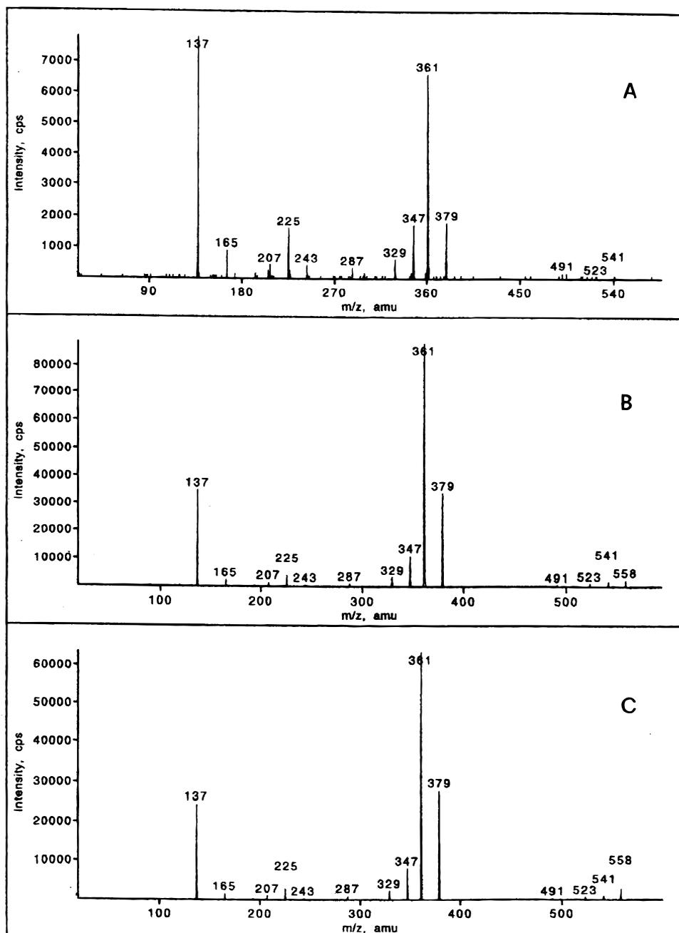
**Figure 2.** ISI tandem mass spectra of oleuropein (1). Product ion spectra (A) from  $[M+H]^+$  and (B) from  $[M+NH_4]^+$  precursors obtained from the commercial standard. Product ion spectrum (C) from  $[M+NH_4]^+$  precursors obtained from the extracted ion chromatogram shown in Fig. 1(B).
