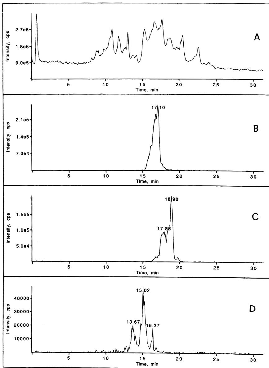
**Figure 1.** (A) Reconstructed ion chromatograms obtained from 20  $\mu$ l of a methanolic extract of young olive leaf from *Olea europaea* L. cv. Cassanese. Total ion current in the range 100–900 units plotted vs. elution time. Extracted ion chromatograms from (B) 558.2 u, (C) 541.2 u and (D) 720.2 u are also shown.
