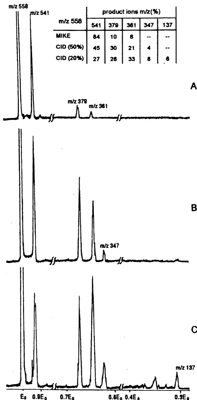
**Figure 3.** FAB tandem mass spectra of  $[M + NH_4]^+$  from oleuropein (1). (A) MIKE and (B) and (C) CID spectra taken at different internal energies of the precursors.
