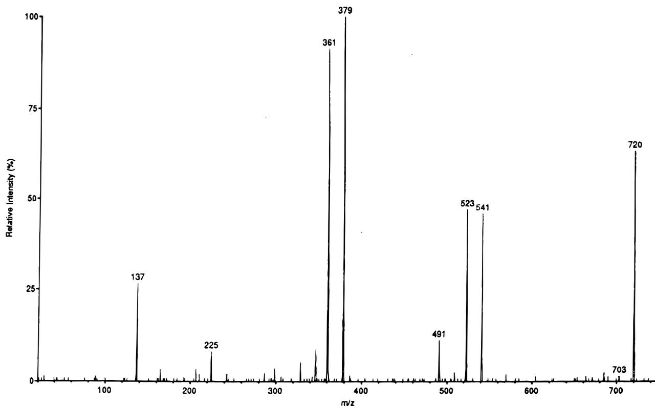
Figure 5. ISI tandem mass spectrum of the  $m/z$  720 ion from the extracted ion chromatogram shown in Fig. 1(D).
